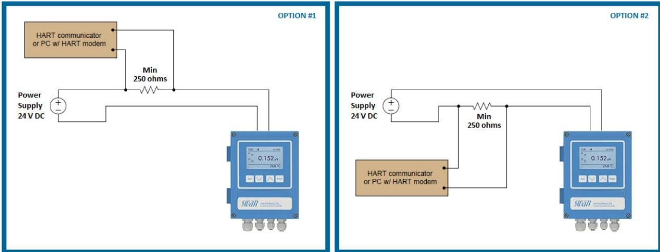
An external minimum  $250 \Omega$  (maximum  $800 \Omega$ ) resistor is needed in order to communicate with HART protocol.
