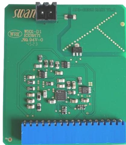
The HARTREC Board must be installed in the AMI-II transmitter in order to communicate with HART.
