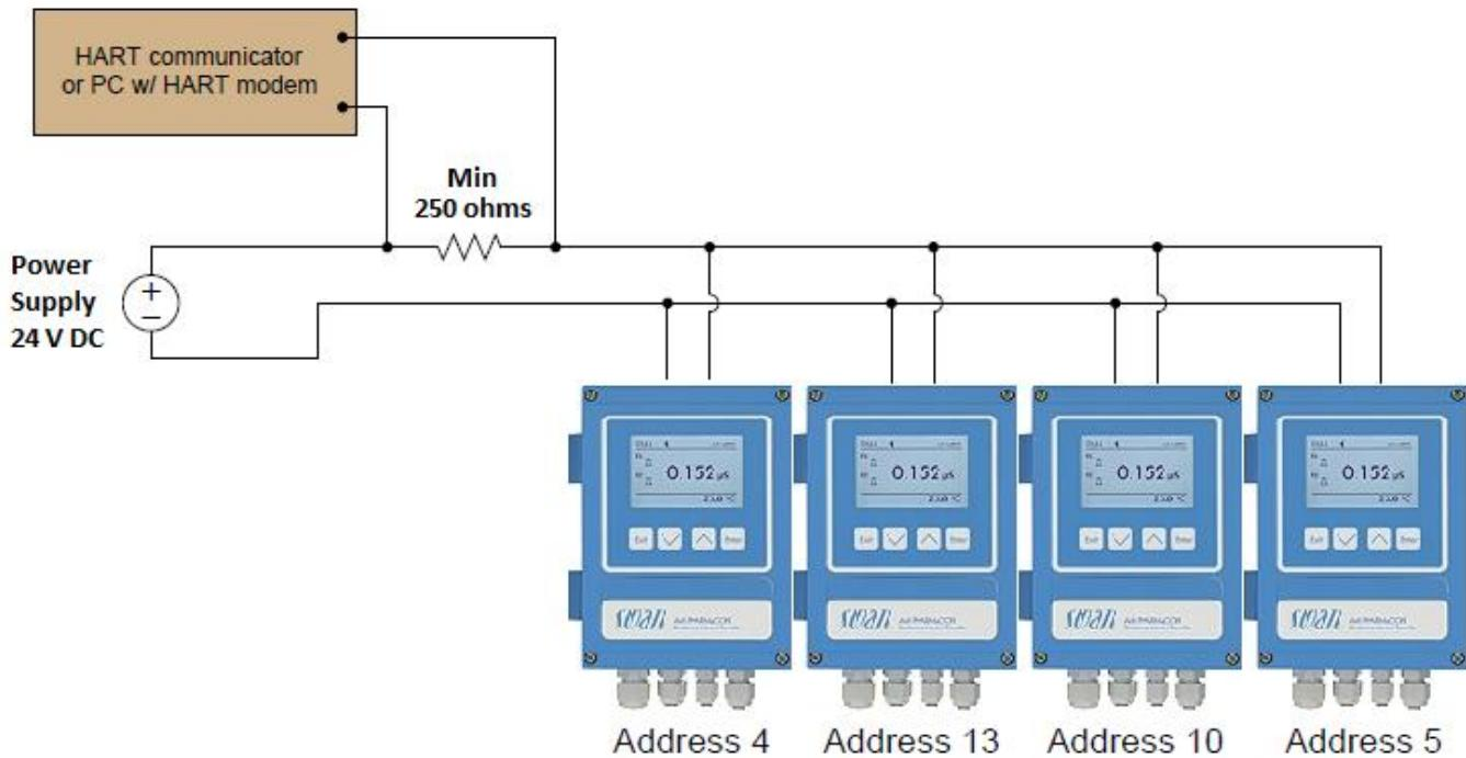
A single minimum  $250 \Omega$  resistor (maximum  $800 \Omega$ ) is needed to communicate with all the instruments connected to the bus, and each of them must provide 4mA.
